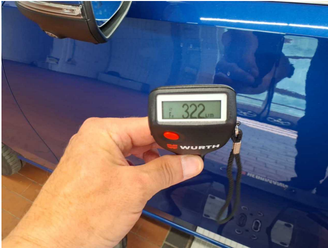
Repainting 5: Door - front left side
