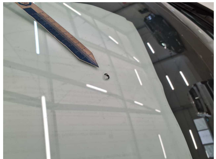
Damage 4: Vehicle glazing: Windscreen - Broken / torn - Replace
