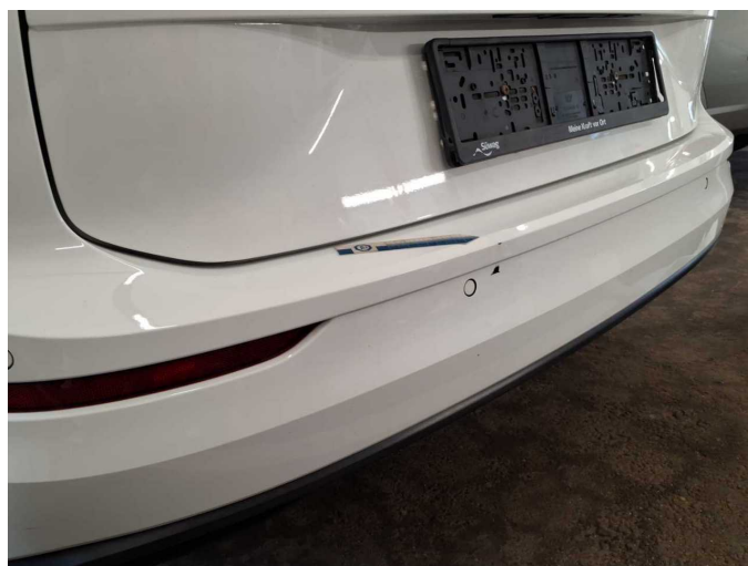
Damage 7: Rear bumper: Rear bumper - Scratched - Paint
