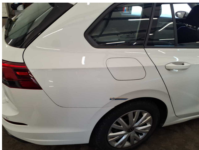
Damage 8: Side panel - rear right side: Side panel (Löcher in Instandgesetzter Fläche) - Paint defect - Repair and paint
