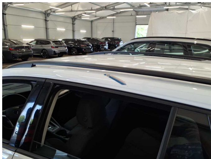
Damage 4: Roof: Roof rail - left side - Scratch(es) - Smart repair
