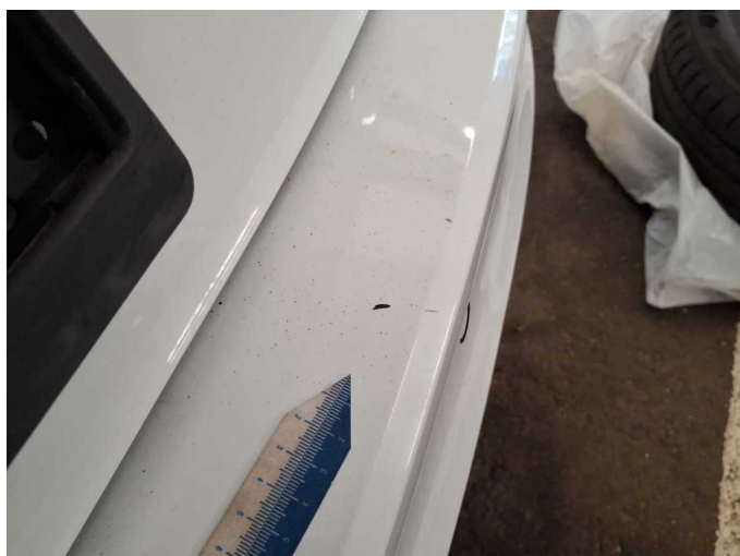
Damage 7: Rear bumper: Rear bumper - Scratched - Paint
