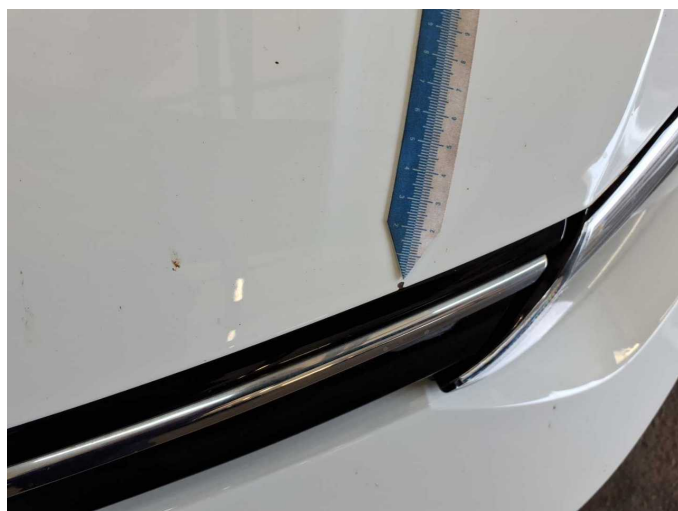
Damage 6: Bonnet: Bonnet - Corrosion - Paint
