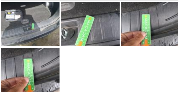
Internal boot lining R, Scratch(es), Acceptable
