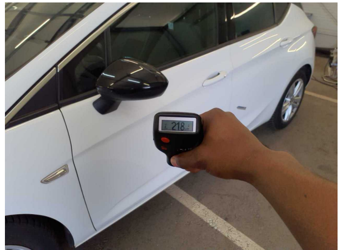
Repainting 4: Door - front left side
