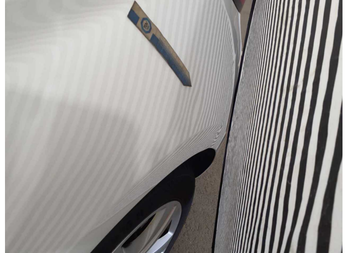
Wear and tear 1: Side panel - rear left side: Side panel - dent(s) - Smooth repair work
