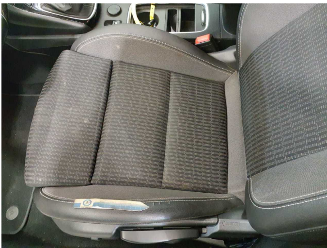
Damage 8: Seat - front: Seat cover - left side - Broken / torn - Smart repair
