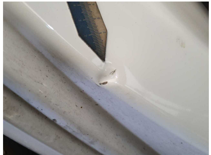
Damage 11: Side panel - rear right side: Sill - Dent / paintcoat damage - Smart repair
