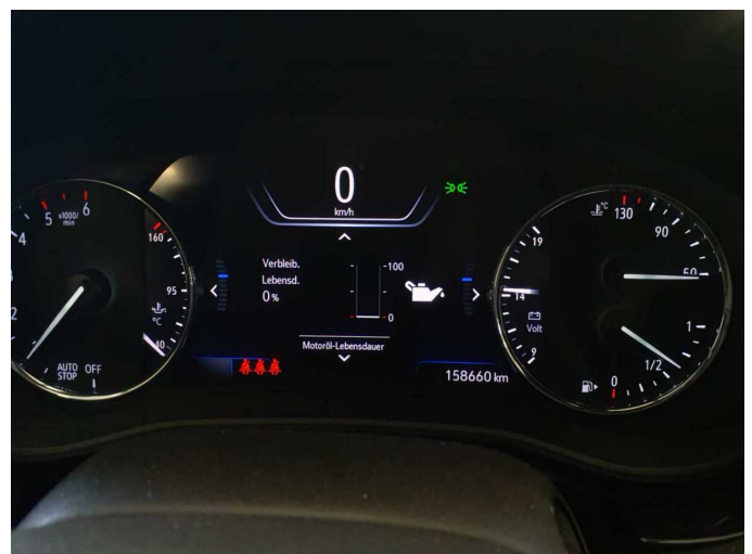
Damage 12: Misc.: Inspection / maintenance - Due - Perform
