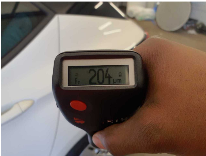
Repainting 3: Side panel - rear left side
