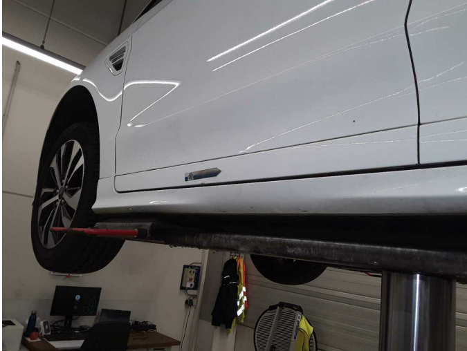
Damage 3: Door - front left side: Brightware - lower - Scratch(es) - Smart repair
