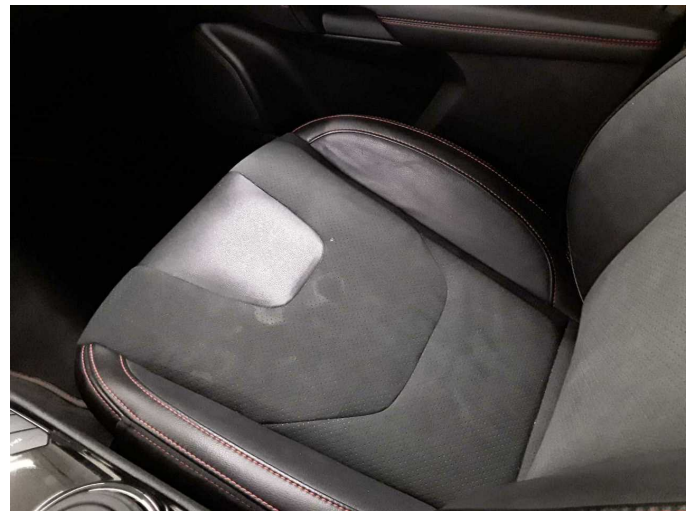
Damage 1: Seat - front: Seat cover - right side - Soiled - Clean
