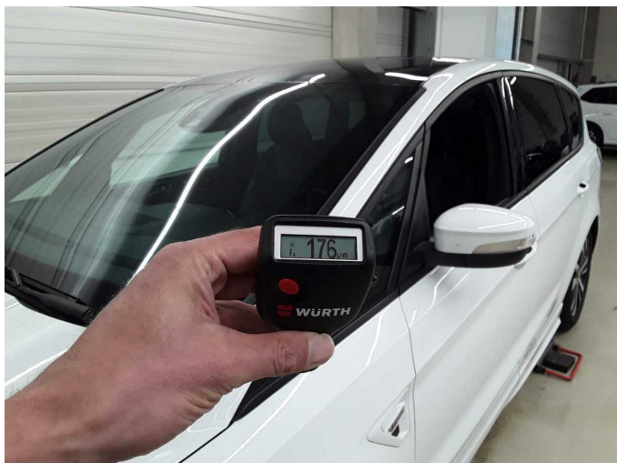
Roof rail - left side: 176 µm
