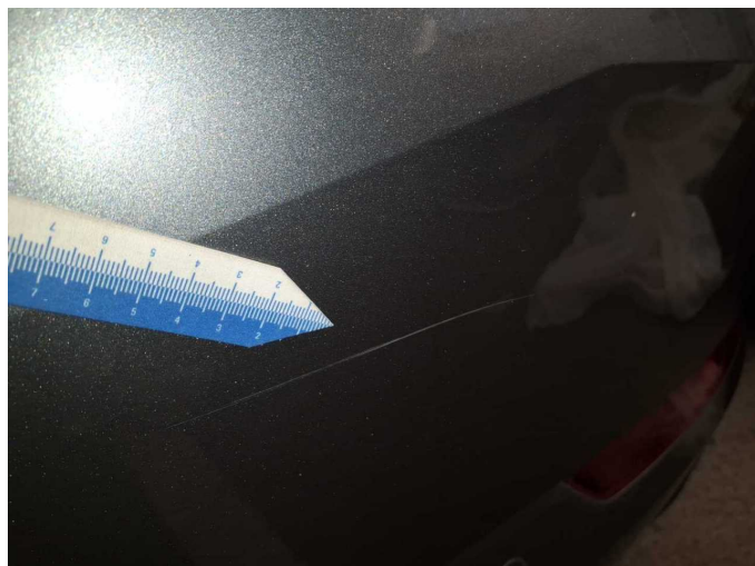
Damage 1: Rear bumper: Rear bumper - Scratch(es) - Paint
