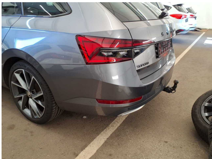
Damage 1: Rear bumper: Rear bumper - Scratch(es) - Paint
