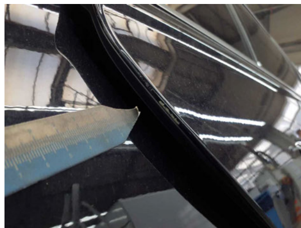
Beschädigung #6: Tür hinten rechts: Tür - Delle / Lackschaden - Smart Repair
