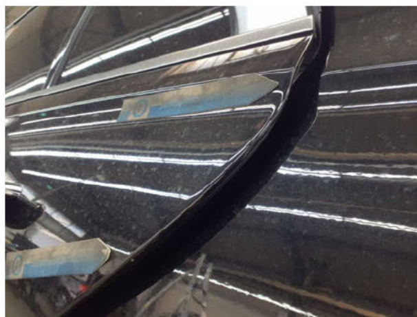
Beschädigung #1: Tür hinten links: Tür - Kratzer - Smart Repair
