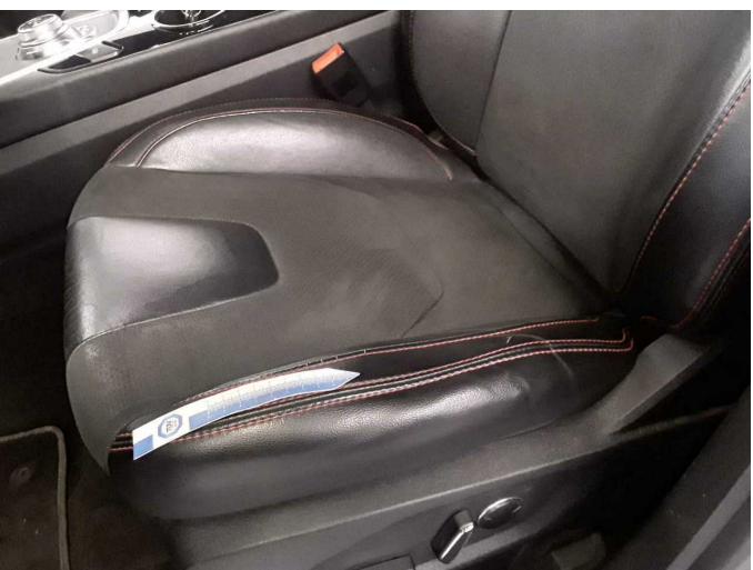
Damage 1: Seat - front: Seat cover - left side - Porous / cracked - Smart repair
