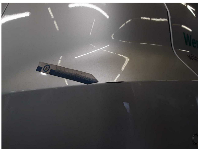
Damage 6: Rear bumper: Rear bumper - Dent / paintcoat damage - Repair and paint
