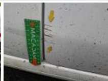
Sliding door R, Dent(s) and scratch(es), Repair and paint (complete)
