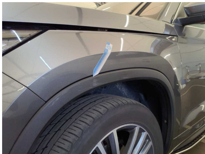
Damage 3: Mudguard - left side: Wheel well extension - Scratch(es) - Replace
