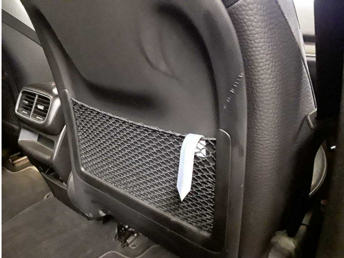
Damage 3: Seat - front: Backrest cover - right side (Lehenschale) - Scratched - Replace
