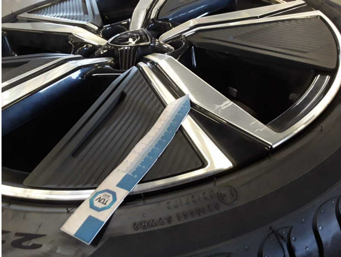
Damage 7: Wheel / tyres: Wheel rims - complete set - Scratch(es) - Loss in value
