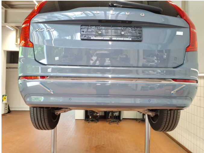
Damage 1: Rear bumper: Rear bumper (Unterteil) - Scratch(es) - Smart repair
