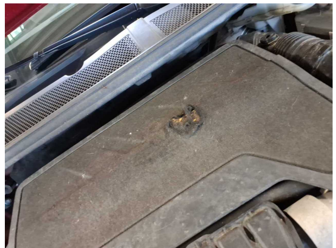
Damage 3: Engine: Engine cover - Damaged - Replace
