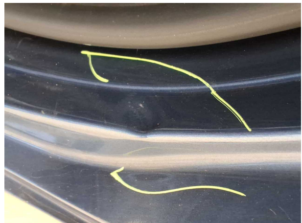
Damage #5: Side panel - rear left side: Sill - dent(s) - Smart repair
