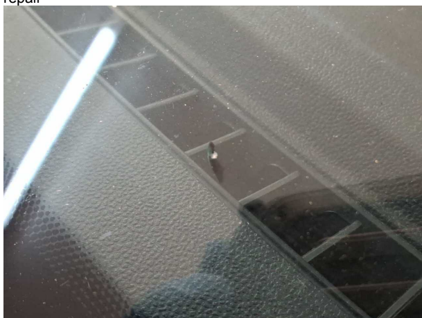
Damage #8: Vehicle glazing: Windscreen - Stone chips - Replace
