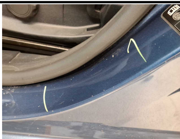
Damage #6: Sill - left side: Sill - Dent / paintcoat damage - Smart repair
