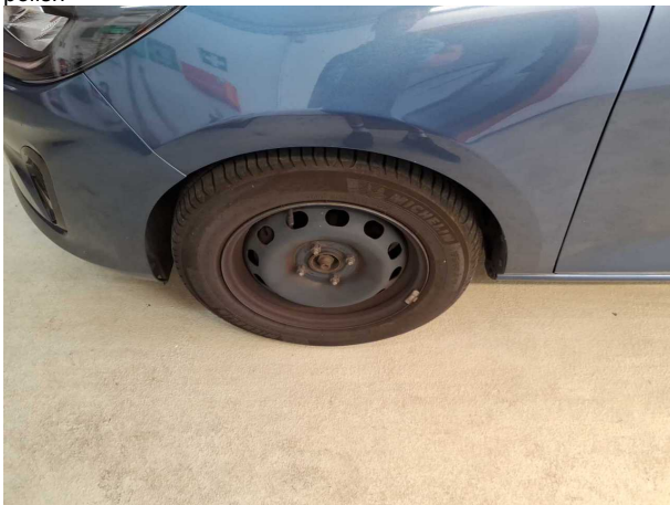
Damage #2: Wheel / tyres: Wheel cover - front left side (Fehlt) - Replace
