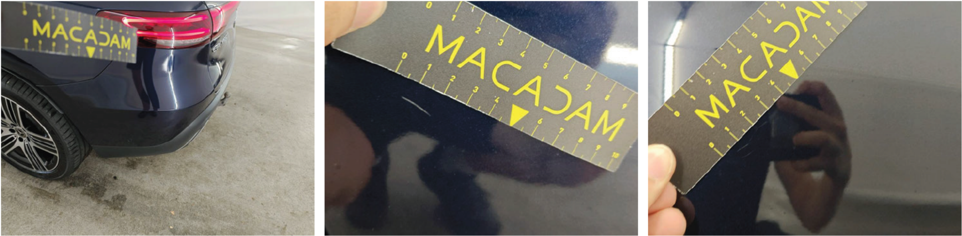
Door RL Scratch(es) Repair and paint (partial) Left
