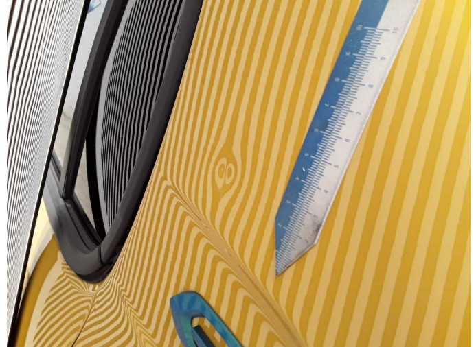
Damage 2: Side panel - rear left side: Side panel - dent(s) - Smart repair
