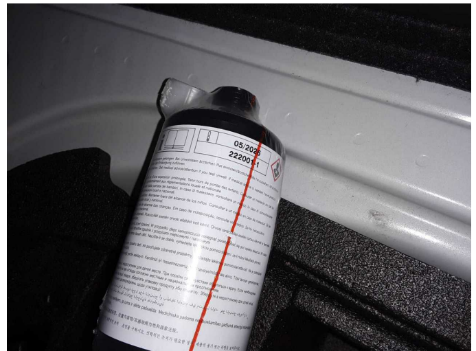
Damage 1: Equipment: Tirefit filler - Due - Replace
