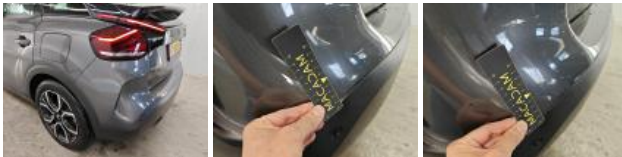
Bumper R, Dent(s) and scratch(es), Repair and paint (complete)
