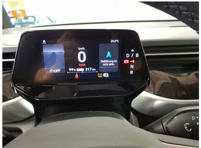
Damage 1: Instrument panel: Indicator light (RDKS) - on - Diagnosed and repair if necessary
