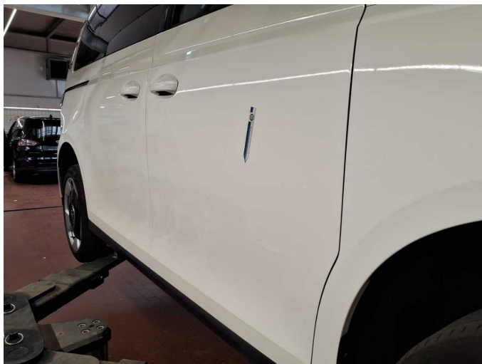
Damage 6: Door - front right side: Door (Orangenhaut) - Unprofessionally repaired - Paint
