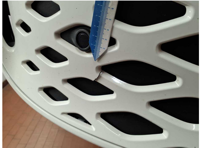
Damage 4: Front bumper: Grille - Broken / torn - Replace
