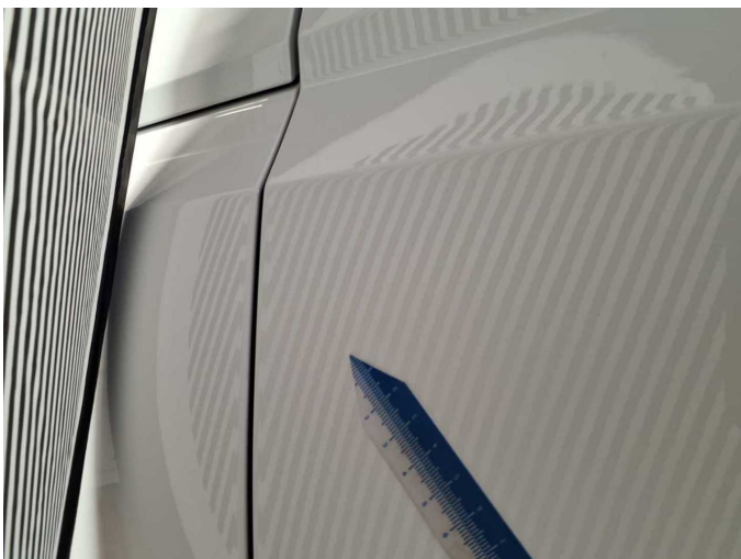
Damage 5: Door - front left side: Door - Unprofessionally repaired - Paint
