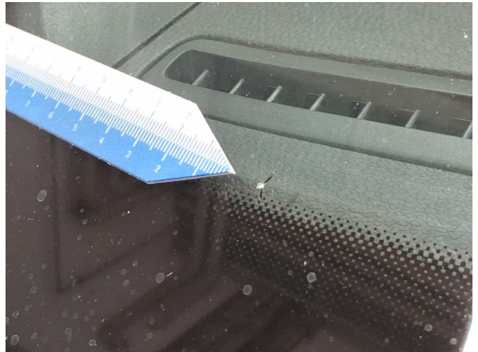
Damage 9: Vehicle glazing: Windscreen - Stone chips - Replace
