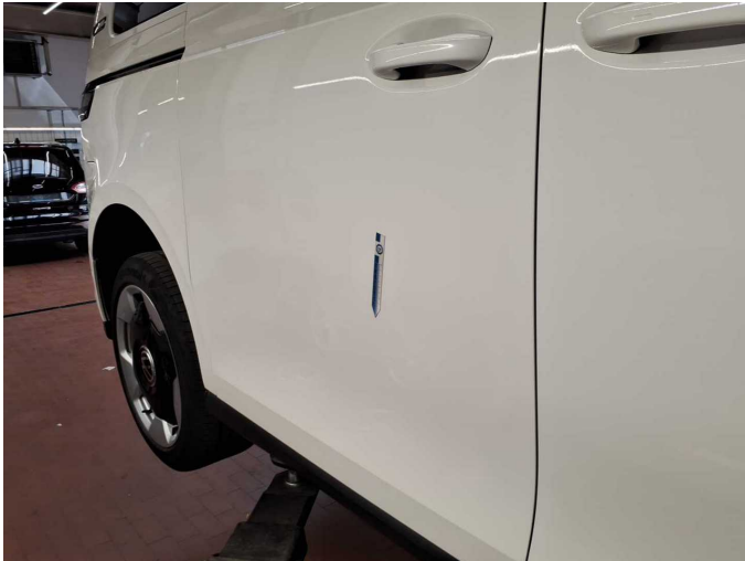
Damage 8: Sliding door, right: Sliding door with glass panel - Unprofessionally repaired - Paint
