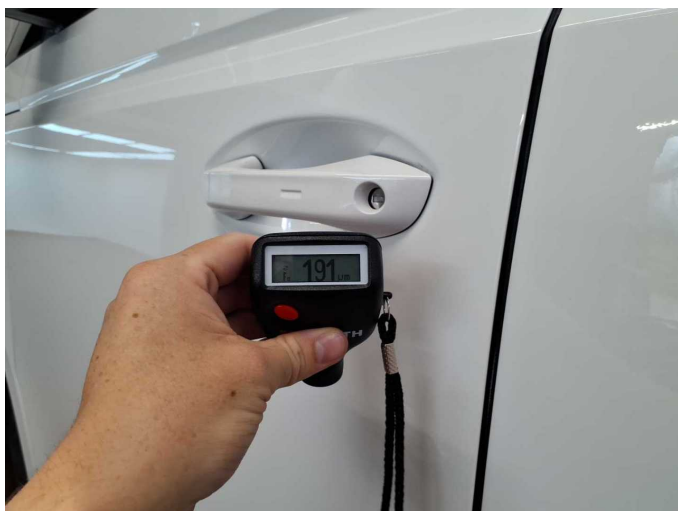
Repainting 4: Door - front left side
