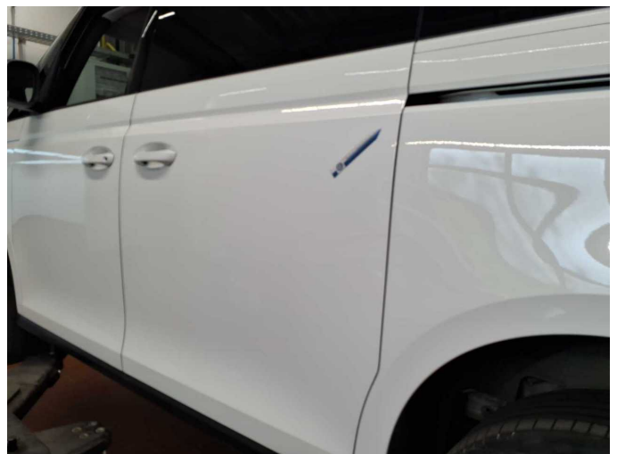
Damage 7: Sliding door - left side: Sliding door with glass panel - Unprofessionally repaired - Paint
