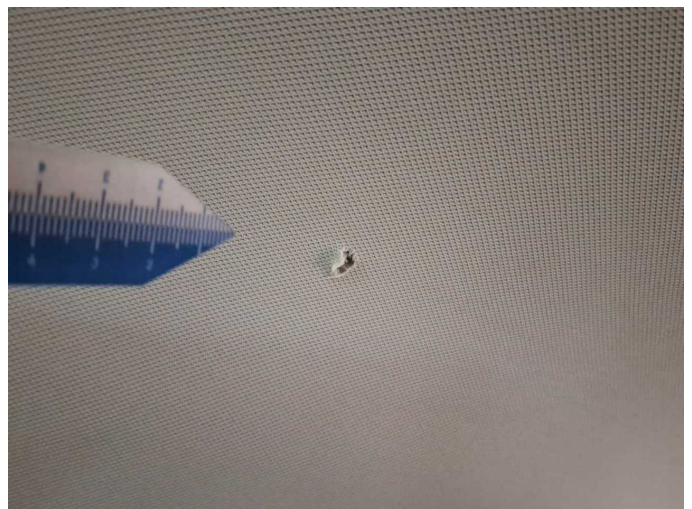
Damage 10: Trim / covers: Roof lining - Broken / torn - Replace
