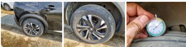
Tyre RL, Out of tolerance, Replace
