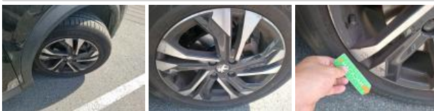
Tyre RR, Out of tolerance, Replace
