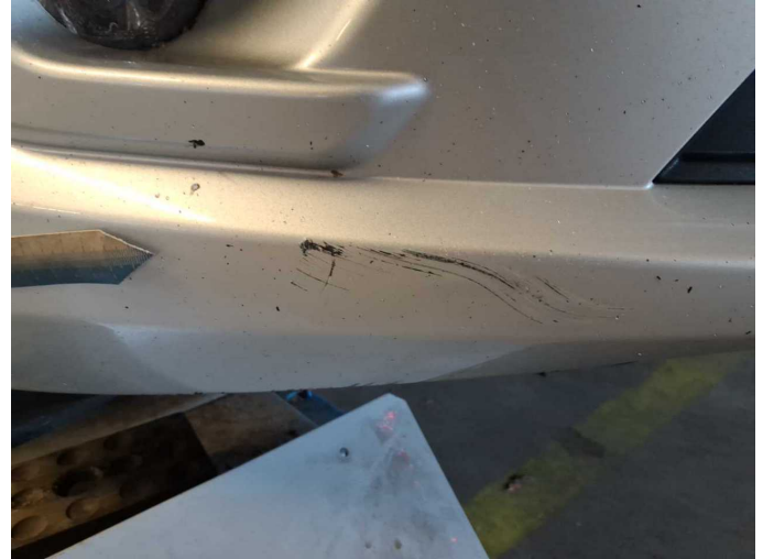
Damage 10: Front bumper: Front bumper - Scratched - Paint
