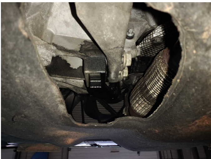
Damage 6: Engine: Engine (Ölfeucht) - Leaking - Perform diagnosis
