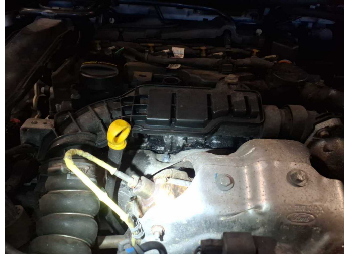
Damage 6: Engine: Engine (Ölfeucht) - Leaking - Perform diagnosis
