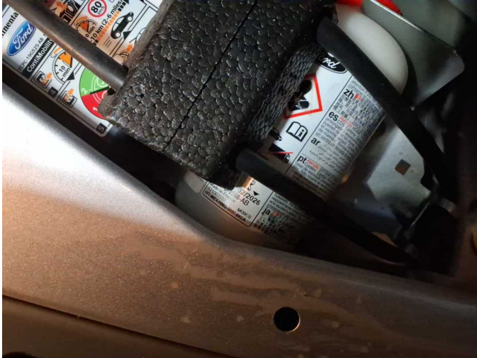
Damage 2: Equipment: Tirefit filler - Expired - Replace
