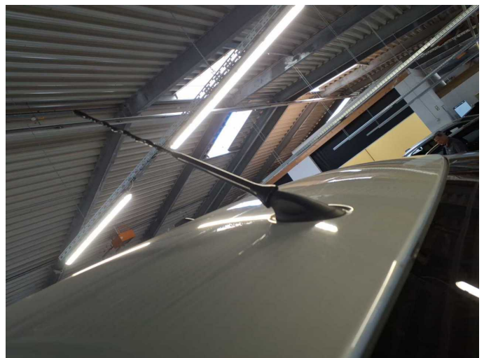
Damage 1: Roof: Stub aerial (Nicht original) - Differs from the original configuration - Replace
