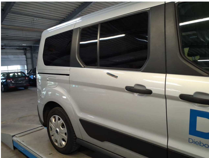
Damage 11: Sliding door, right: Sliding door with glass panel - Deformed - Repair and paint
