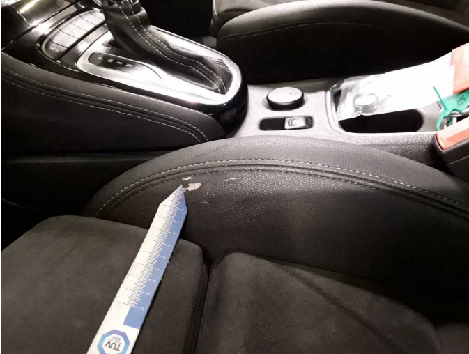
Damage 5: Seat - front: Seat cover - left side - Scratched - Smart repair
