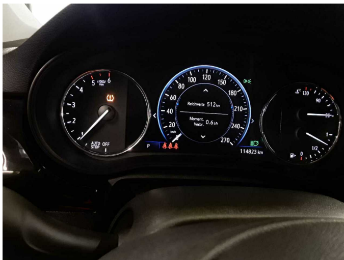
Damage 4: Wheel / tyres: Pressure sensor (Reifendruck) - on - Perform diagnosis
