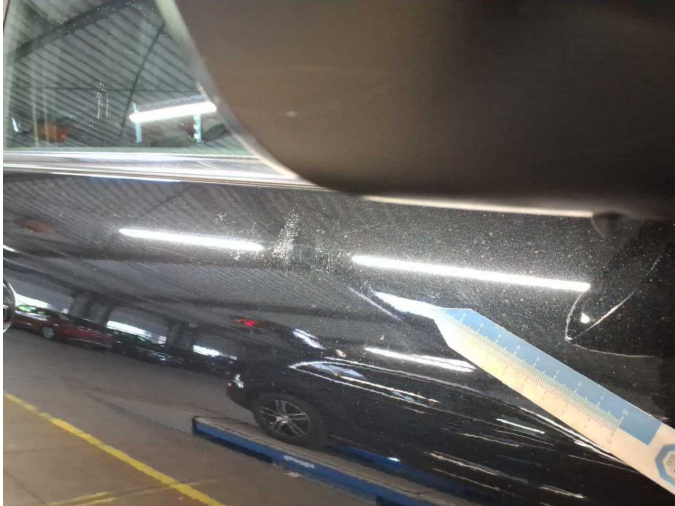
Damage 8: Door - front right side: Door (Einschlüsse, dellen) - Unprofessionally repaired - Repair and paint
