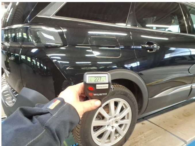
Repainting 2: Side panel - rear right side
