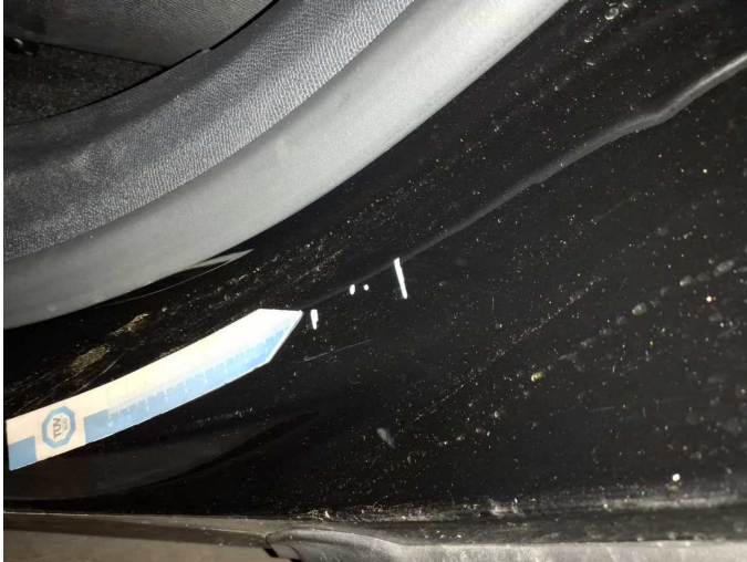
Damage 6: Side panel - rear left side: Sill - Dent / paintcoat damage - Smart repair
