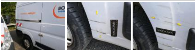
Central pillar moulding R, Missing, Replace
