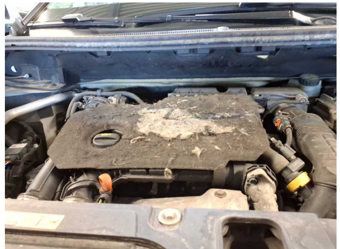
Damage 5: Engine: Engine cover (Evtl Mehrkosten) - Damage caused by marten / rodent - Replace
