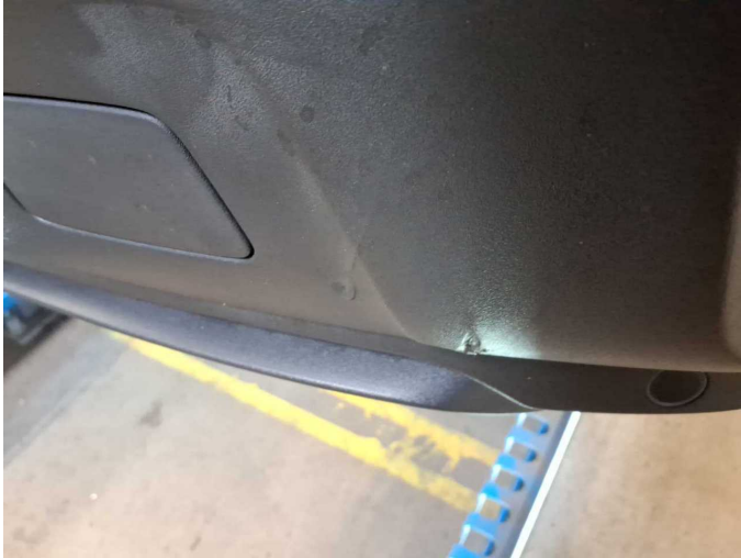
Damage 6: Rear bumper: Rear bumper (unpainted) - Broken / torn - Replace
