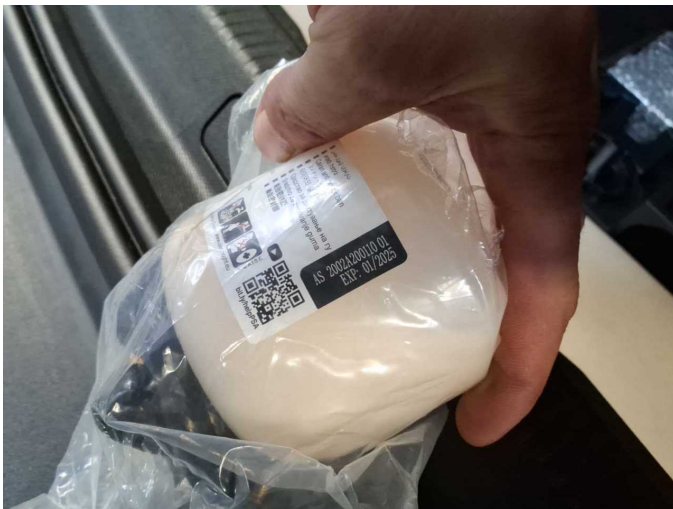
Damage 1: Equipment: Tirefit filler - Expired - Replace
