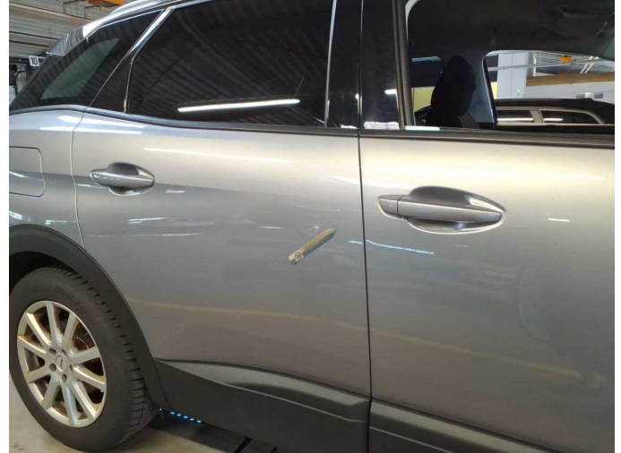
Damage 4: Door - rear right side: Door - Scratch(es) - Smart repair
