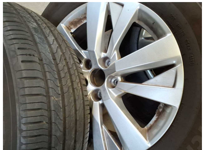
Missing part 1: 2nd wheel set: 1 wheel cover (Nabendeckel) - Missing - Replace
