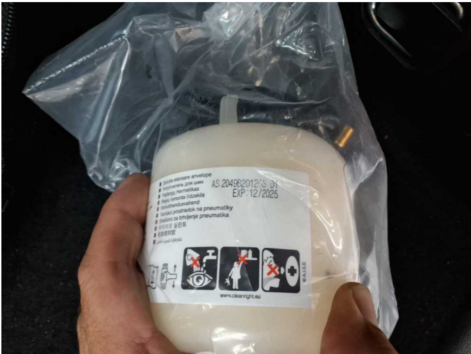
Damage 2: Equipment: Tirefit filler - Expired - Replace
