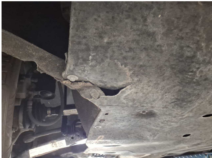
Damage 7: Body: Underbody panelling - Broken / torn - Replace
