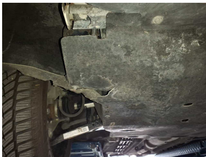
Damage 7: Body: Underbody panelling - Broken / torn - Replace
