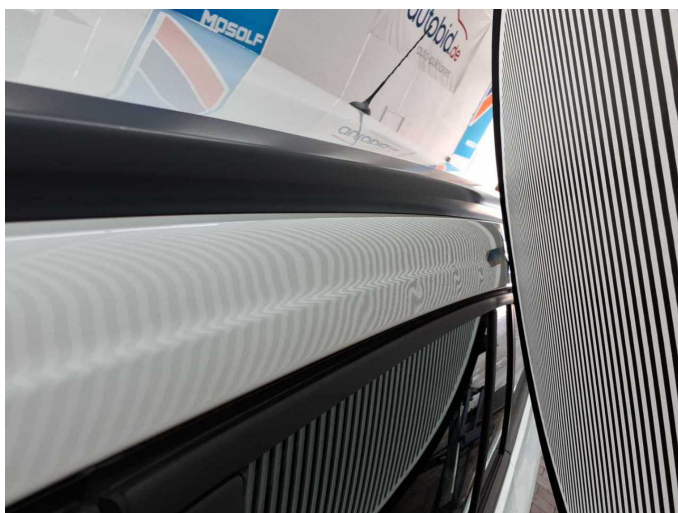
Damage 8: Roof: Roof rail - left side - dent(s) - Smooth repair work
