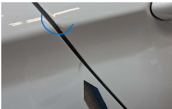
Damage 6: Door - rear right side: Door - Scratch(es) - Smart repair
