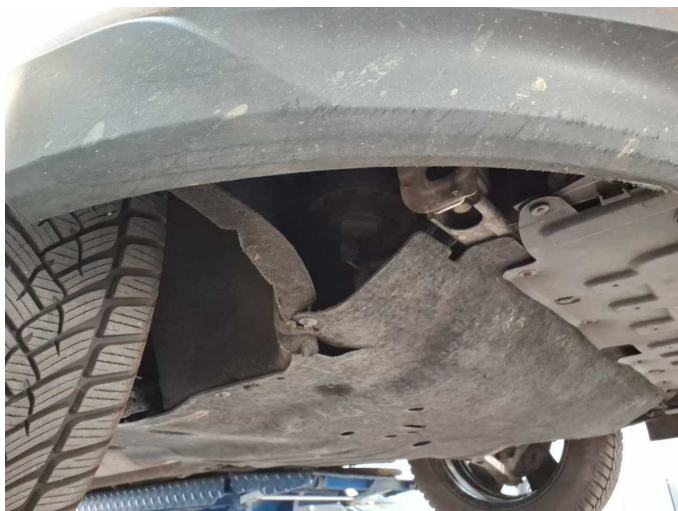
Damage 4: Side panel - rear right side: Wheel arch (Radhausschale) - Broken / torn - Replace
