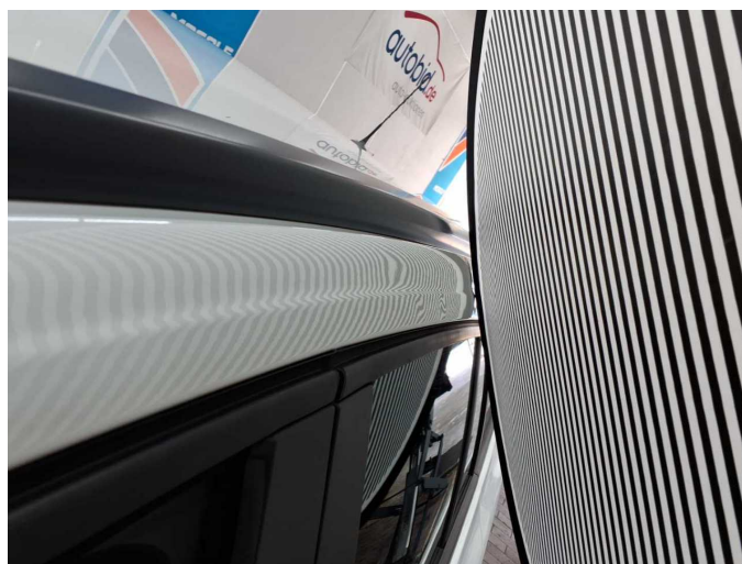
Damage 8: Roof: Roof rail - left side - dent(s) - Smooth repair work
