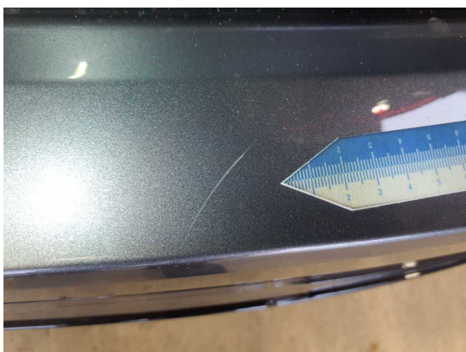
Damage 2: Rear bumper: Rear bumper - Scratch(es) - Paint
