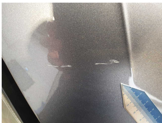
Damage 3: Bonnet: Bonnet - Dent / paintcoat damage - Repair and paint
