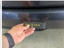
Parking sensor R, Deformed / Strained, Replace
