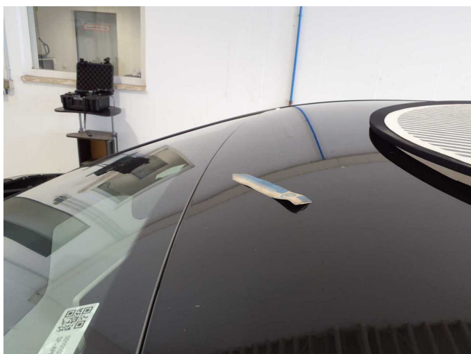
Damage 1: Roof: Roof - dent(s) - Smooth repair work
