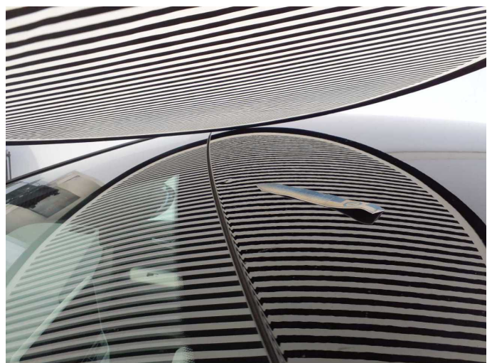
Damage 1: Roof: Roof - dent(s) - Smooth repair work
