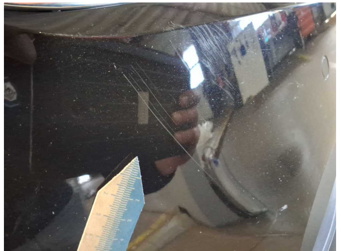
Damage 7: Front bumper: Front bumper - Scratched - Paint
