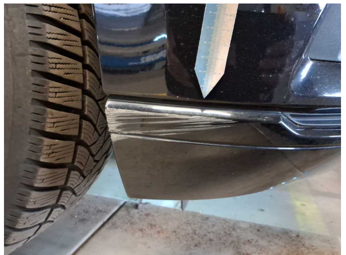
Damage 7: Front bumper: Front bumper - Scratched - Paint
