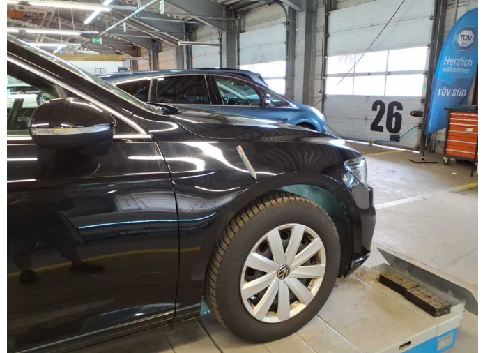
Damage 6: Mudguard - right side: Mudguard - right side - Dent / paintcoat damage - Smart repair
