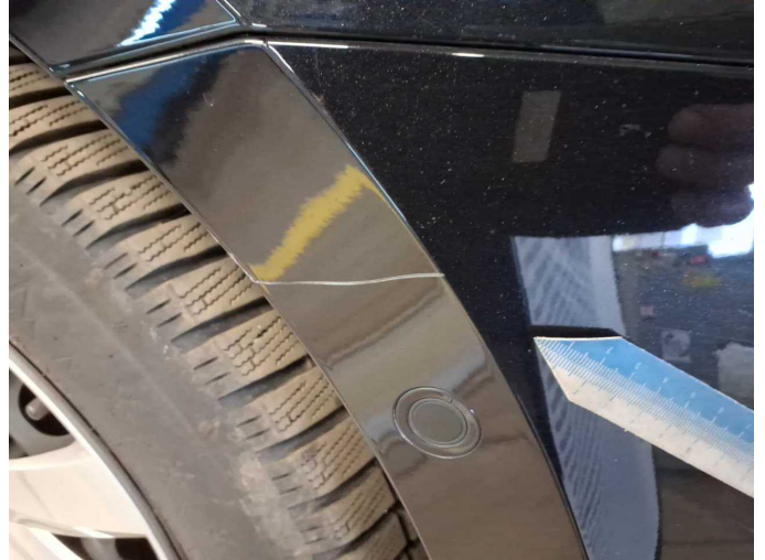
Damage 7: Front bumper: Front bumper - Scratched - Paint
