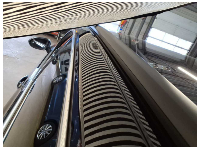
Damage 5: Roof: Roof rail - left side - dent(s) - Smooth repair work
