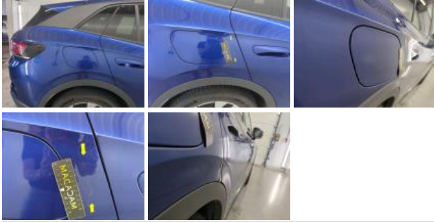
Fuel cap cover, Scratch(es), Repair and paint (complete)
