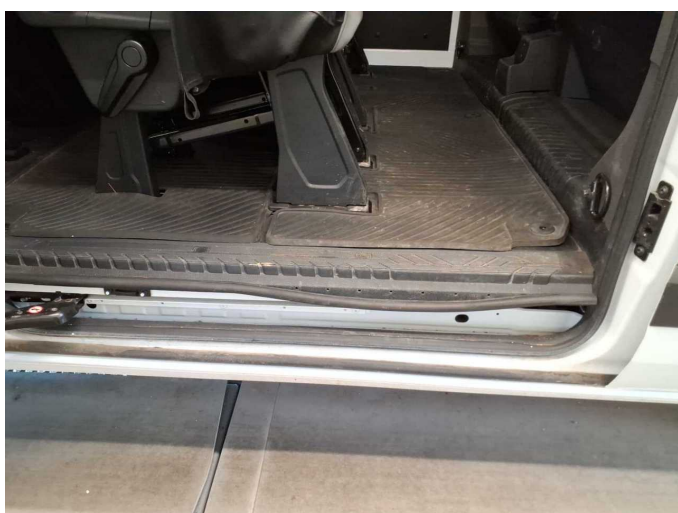
Damage 2: Sliding door, right: Door seal - Loose - Repair
