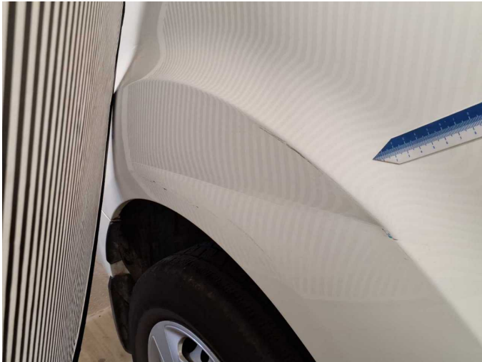
Damage 5: Side panel - rear right side: Side panel (Unterhalb) - Dent / paintcoat damage - Repair and paint
