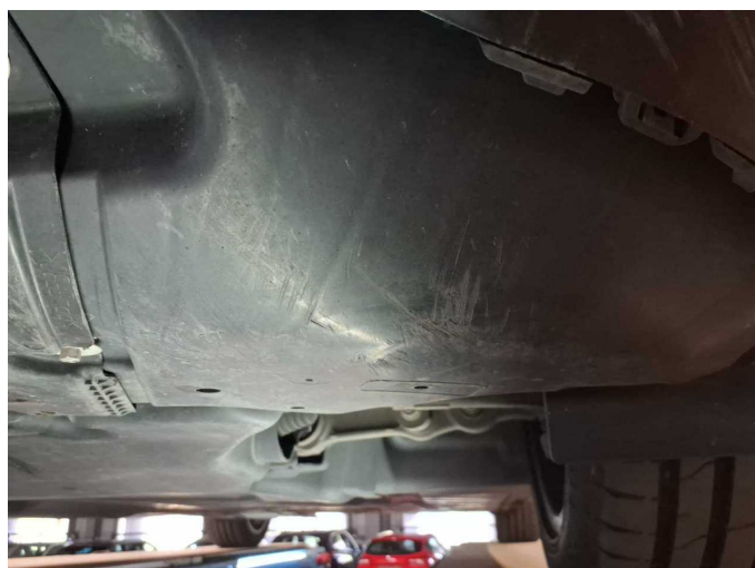
Damage 5: Body: Underbody panelling - Scratch(es) - Replace
