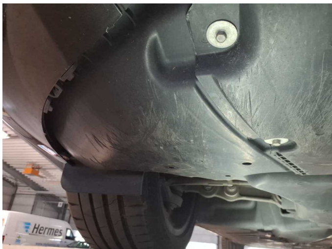
Damage 5: Body: Underbody panelling - Scratch(es) - Replace
