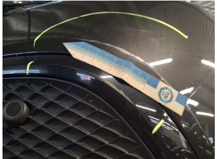
Damage 6: Front bumper: Front bumper (+ Blende) - Scratched - Paint
