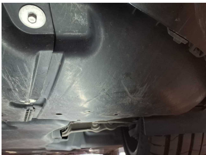
Damage 5: Body: Underbody panelling - Scratch(es) - Replace
