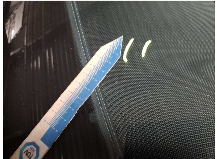
Wear and tear 2: Vehicle glazing: Windscreen - Stone chips
