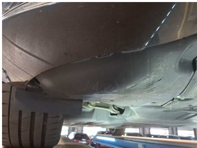
Damage 5: Body: Underbody panelling - Scratch(es) - Replace
