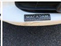
Boot lid covering R, Scratch(es), Replace
