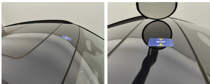
Roof // Smart Repair Medium-dent
