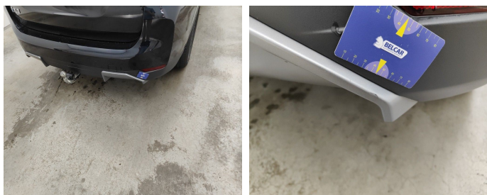
Bumper Rear / Trim Right / Replace-scratch + dent
