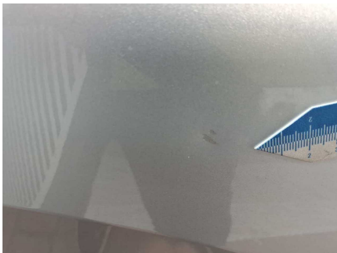
Damage 3: Side panel - rear left side: Side panel - Dent / paintcoat damage - Paint
