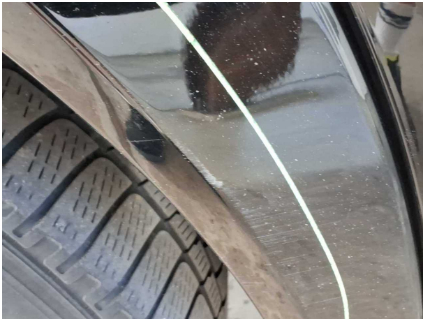
Damage #6: Side panel - rear right side: Wheel well extension - Scratched - Smart repair
