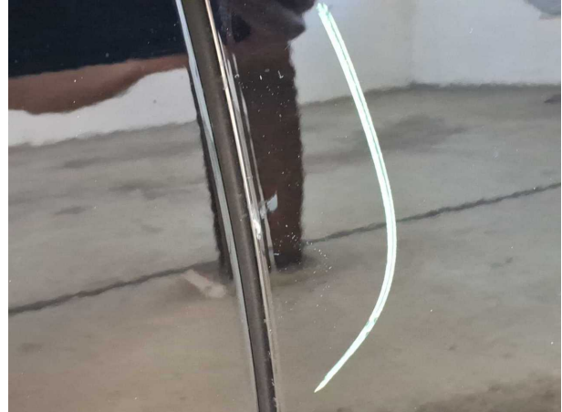
Damage #2: Door - front right side: Door edge - Scratched - Cover / polish
