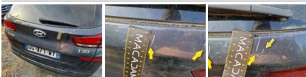
Bumper R, Broken, Replace and paint
