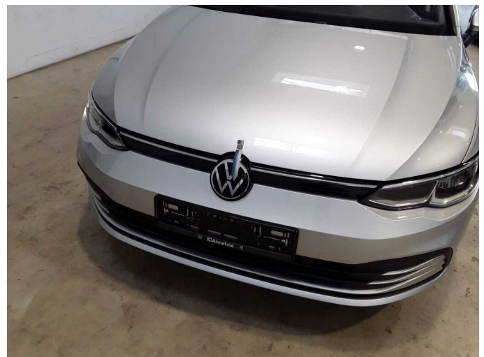
Damage 5: Front structure: Emblem - Broken / torn - Replace
