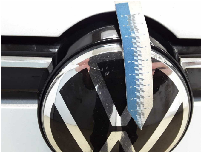
Damage 5: Front structure: Emblem - Broken / torn - Replace
