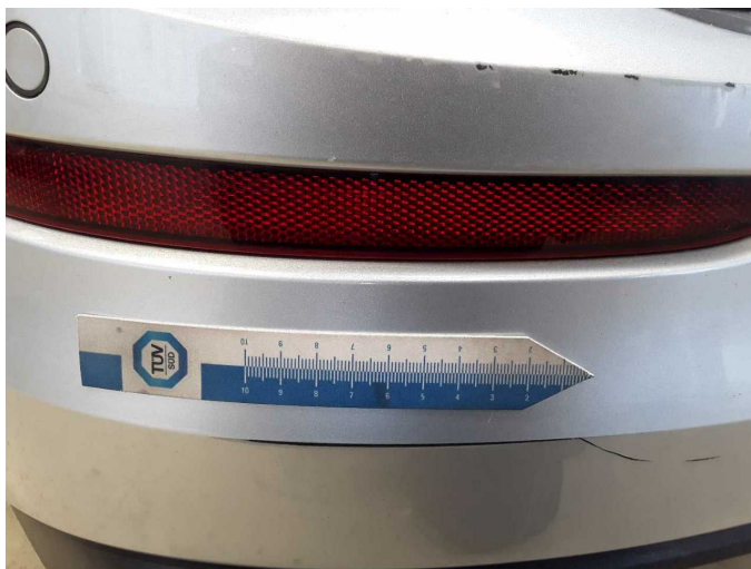
Damage 8: Rear bumper: Rear bumper - Scratch(es) - Paint
