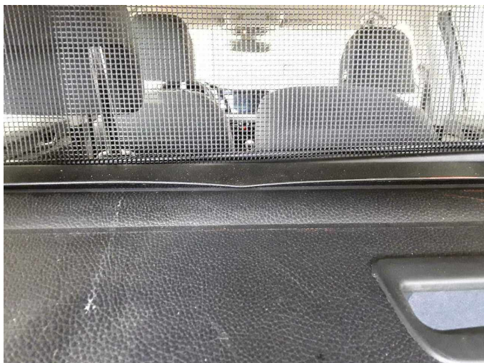
Wear and tear 1: Interior: Boot cover / roller cover - Deformed - No deduction
