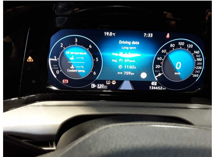
Damage 2: Instrument panel: Indicator light (Reifendruck) - on - Perform diagnosis
