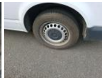
Tyre RR, Out of tolerance, Replace
