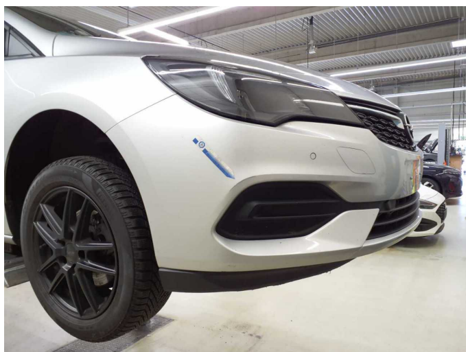
Damage 3: Front bumper: Bumper with Parktronic - Scratched - Smart repair
