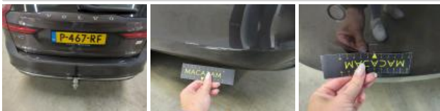
Bumper R, Scratch(es), Repair and paint (complete)
