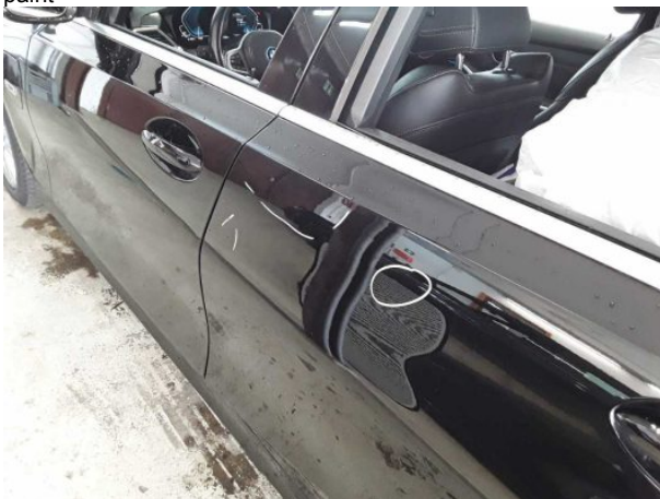
Damage #6: Door - rear left side: Door - Dent / paintcoat damage - Repair and paint
