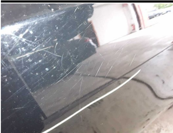
Damage #6: Door - rear left side: Door - Dent / paintcoat damage - Repair and paint
