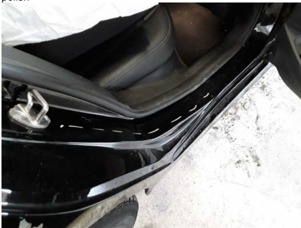
Damage #3: Side panel - rear right side: Sill - Scratched - Repair and paint
