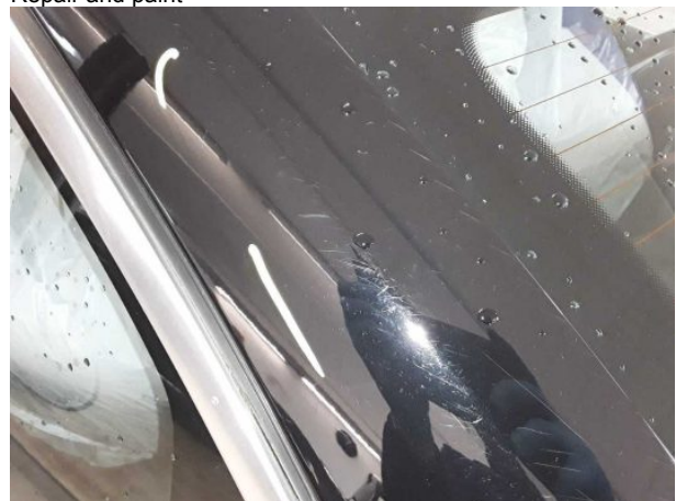
Damage #4: Roof: Roof rail - left side - Scratched - Paint
