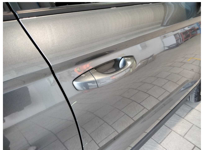
Damage 4: Door - front right side: Door handle - outside - Scratch(es) - Smart repair
