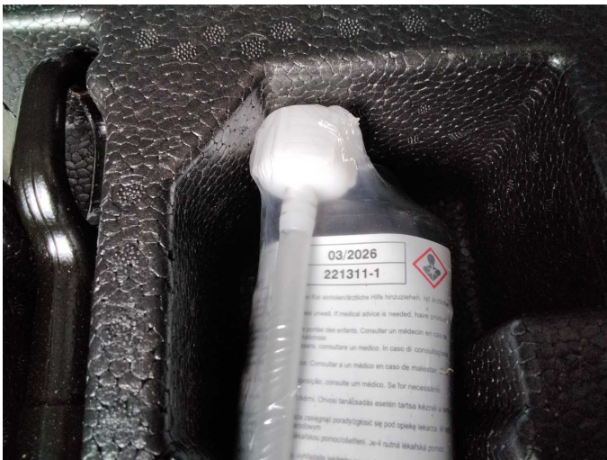
Damage 2: Equipment: Tirefit filler - Expired - Replace
