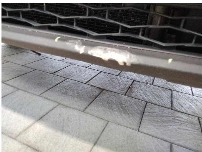
Damage 9: Front bumper: Spoiler - Deformed - Replace
