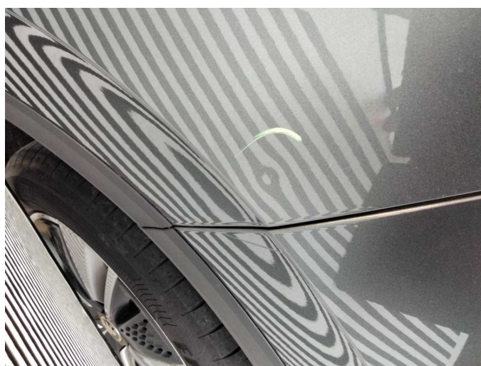
Damage 8: Side panel - rear left side: Side panel (+ Kratzer Gebrauchsspur) - dent(s) - Smart repair
