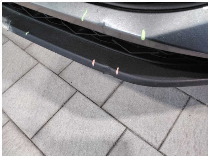
Damage 9: Front bumper: Spoiler - Deformed - Replace
