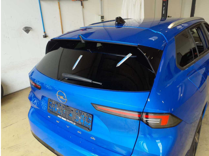
Damage 3: Vehicle glazing: Rear window - Scratch(es) - Replace
