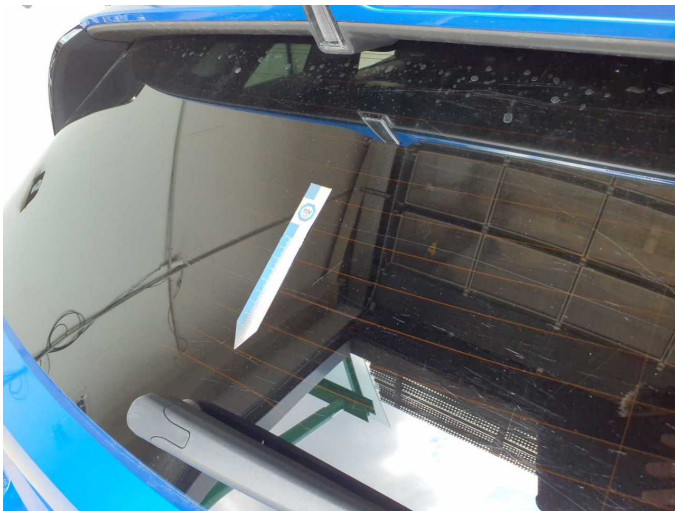
Damage 3: Vehicle glazing: Rear window - Scratch(es) - Replace
