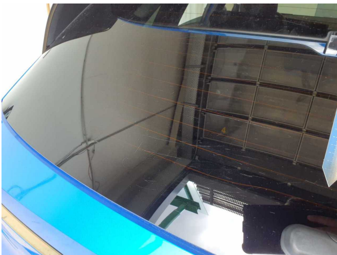
Damage 3: Vehicle glazing: Rear window - Scratch(es) - Replace
