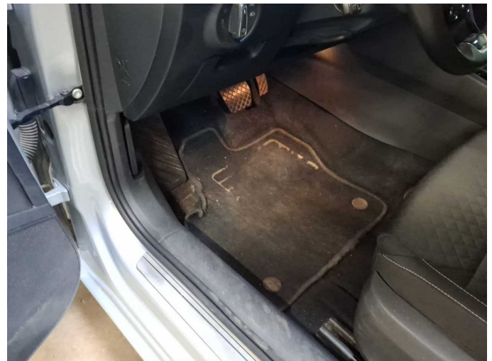
Damage 1: Trim / covers: Floor mats - Deformed - Replace
