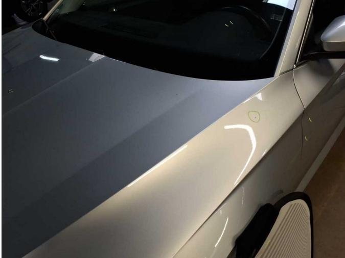
Damage 7: Bonnet: Bonnet - Stone chips - Paint
