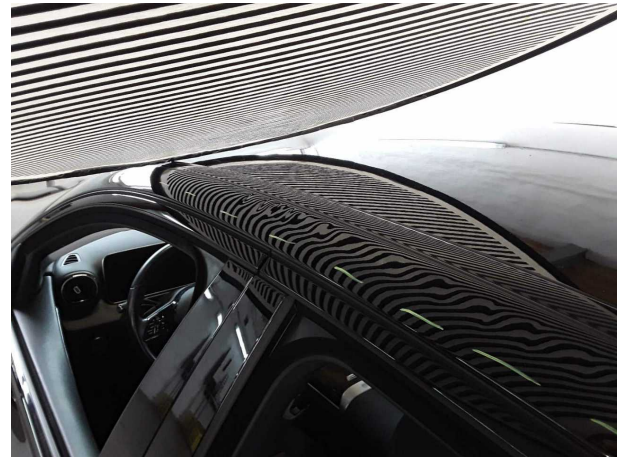
Damage #4: Roof: Roof rail - left side - Dent / paintcoat damage - Repair and paint
