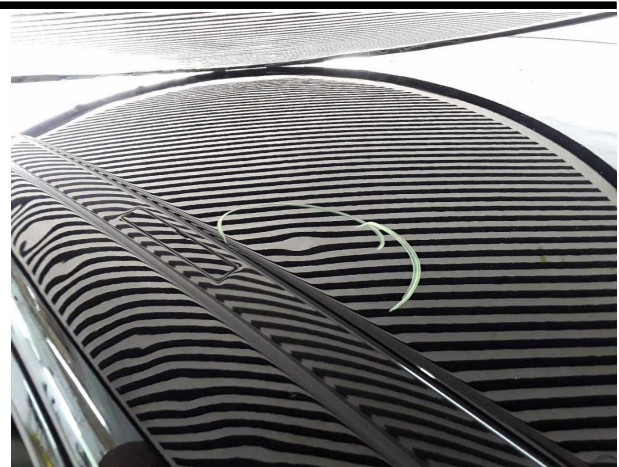
Damage #3: Roof: Roof (2 Stück) - dent(s) - Smooth repair work
