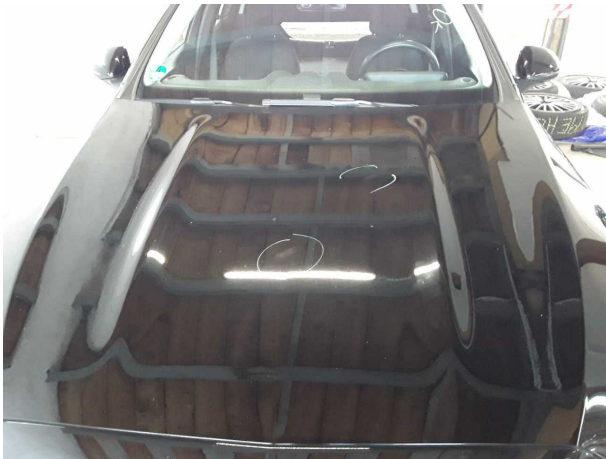
Damage #1: Bonnet: Bonnet - Scratched - Cover / polish
