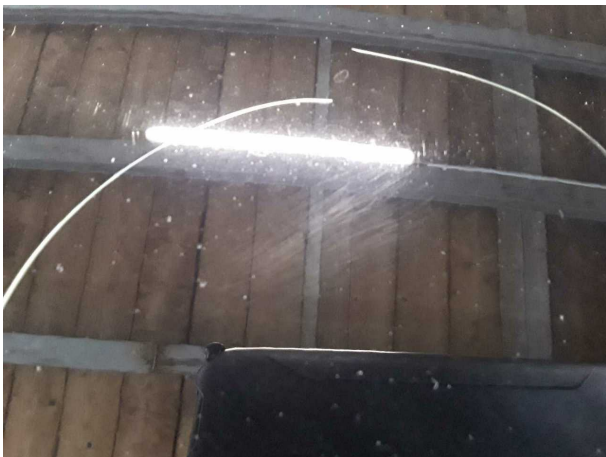
Damage #1: Bonnet: Bonnet - Scratched - Cover / polish
