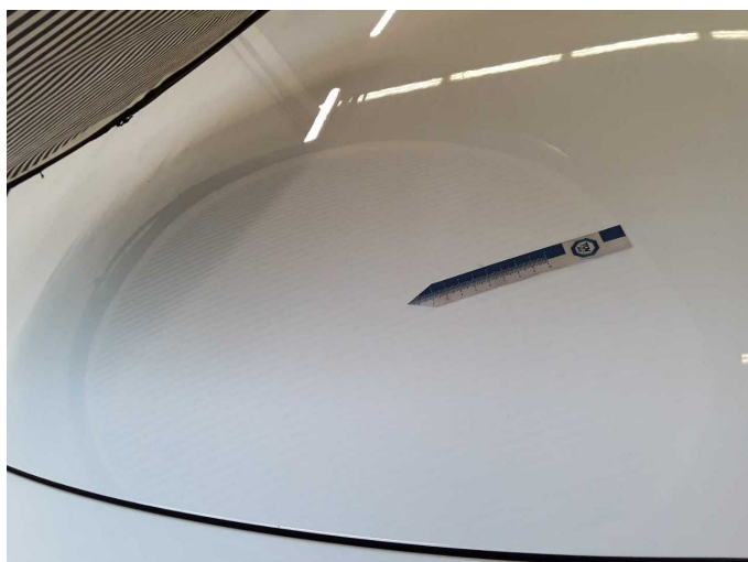
Damage 1: Bonnet: Bonnet - dent(s) - Smooth repair work
